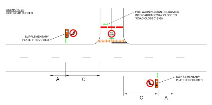
In speed environments greater than 65kph, or where major risks exist (eg tight geometrics, restricted visibility, narrow road carriageway etc), then STMSs must enhance or extend warning signage on the main road approaches to provide sufficient warning. This may require deploying the normal F2:25 layout.
