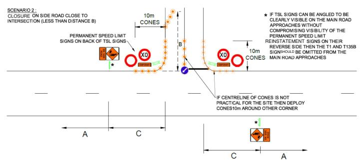
Where significant hazards exist on the sideroad close to the main road intersection, then STMSs must enhance or extend signage on the main road approaches to provide sufficient warning. This may require deploying the normal F2:20 layout.
