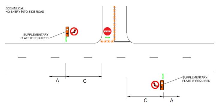
In speed environments greater than 65kph, or where major risks exist (eg tight geometrics, restricted visibility, narrow road carriageway, rough / unsealed surface etc), then STMSs must enhance or extend warning signage on the main road approaches to provide sufficient warning. This may require deploying the normal F2:25 layout.
